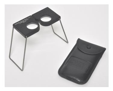
The #758 Stereo Viewer is a folding, pocket sized viewer which is ideal for three dimensional viewing of stereomicrographs. The precision ground and coated lenses give a two times magnification. A simple interpupillary adjustment calibrated in millimeters is provided. The viewer is packed in a protective carrying case.
